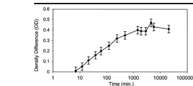
**Figure 3.** Graph shows differences in optical density (OD) over time. Consistent amounts of UV protectants were applied to a  $YTaO_4$  intensifying screen and then cleaned off after varying lengths of time. The optical density difference was measured for each of the artifacts produced.
