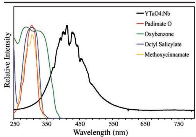
Figure 6. Spectroscopic image shows that the absorbance range of the UV filters overlaps the tail of the  $YTaO_4:Nb$  phosphor emission spectrum.
