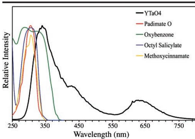
Figure 5. Spectroscopic image shows that the absorbance range of the UV filters overlaps considerably with the emission spectrum of  $YTaO_4$  phosphor.
