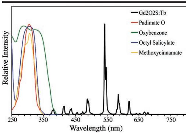
Figure 4. Spectroscopic image shows that the absorbance range of the UV filters does not substantially overlap the emission spectrum of  $Gd_2O_2S:Tb$  phosphor.
