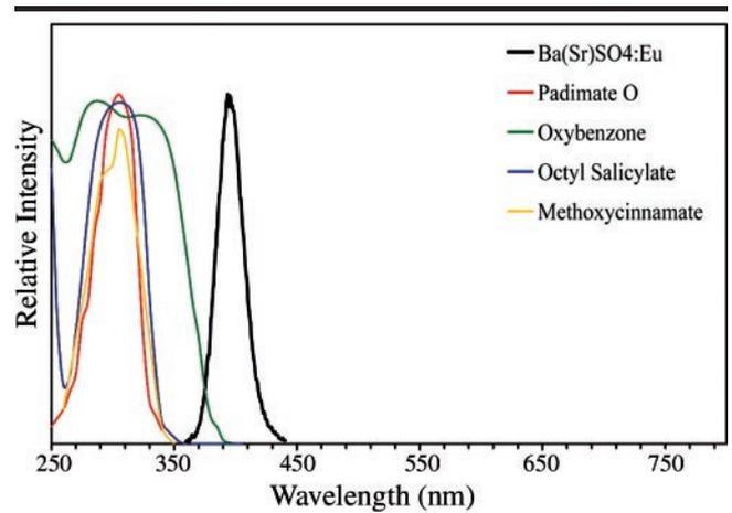
Figure 7. Spectroscopic image shows that the absorbance range of the UV filters overlaps the tail of the  $Ba(Sr)SO_4:Eu$  phosphor emission spectrum.
