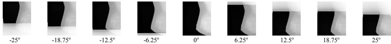
Fig. 2. An example of tomosynthetic acquisition with 9 source projection images, each 6.25 degrees apart. The 0° degree angle corresponds to the central source projection (CSP) image.
