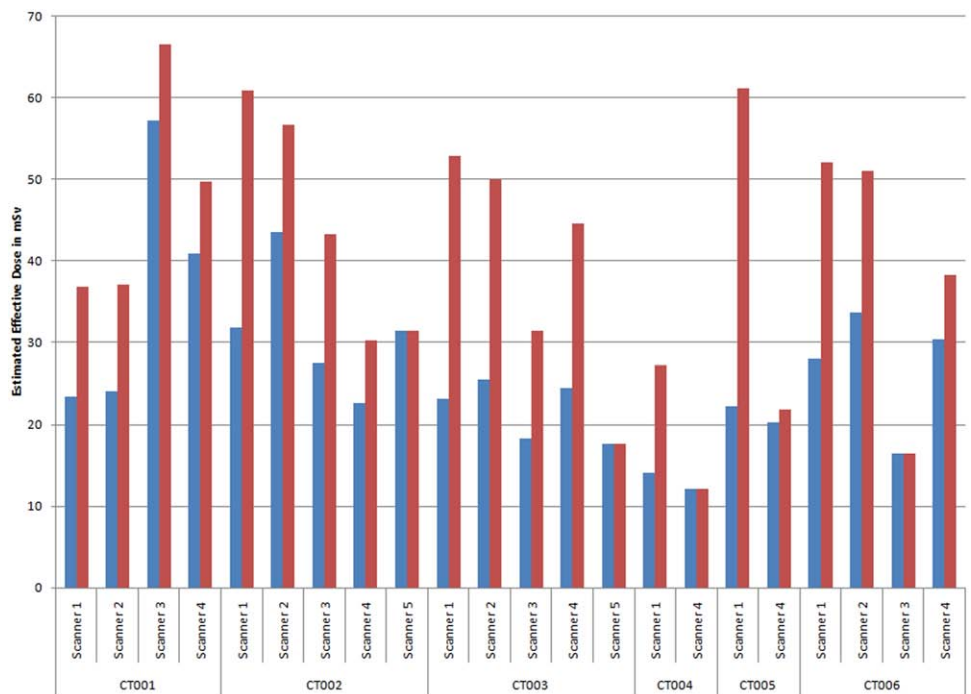
Fig 4. Radiation dose estimate (in millisieverts) during January and February 2010 on different scanner models according to examination type. Columns in blue online (light gray in print) indicate average dose and red columns online (dark gray in print) indicate maximum dose for a particular examination type on a particular scanner model. This analysis can identify protocol issues that can potentially be leading to higher doses (eg, dose estimate on scanners 1 and 2 for examination code CT001 vs for scanners 3 and 4).
