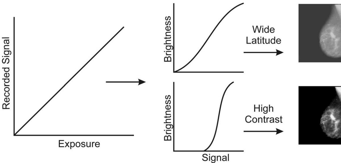
**Fig 2.** An example of the acquisition and display characteristics of a digital imaging system. The recorded signal is linear with exposure. Thus, if the exposure is doubled, the signal is doubled too. The signal is then mapped through a “look-up table” to determine how the image is displayed. Two examples of possible display parameters are shown.
