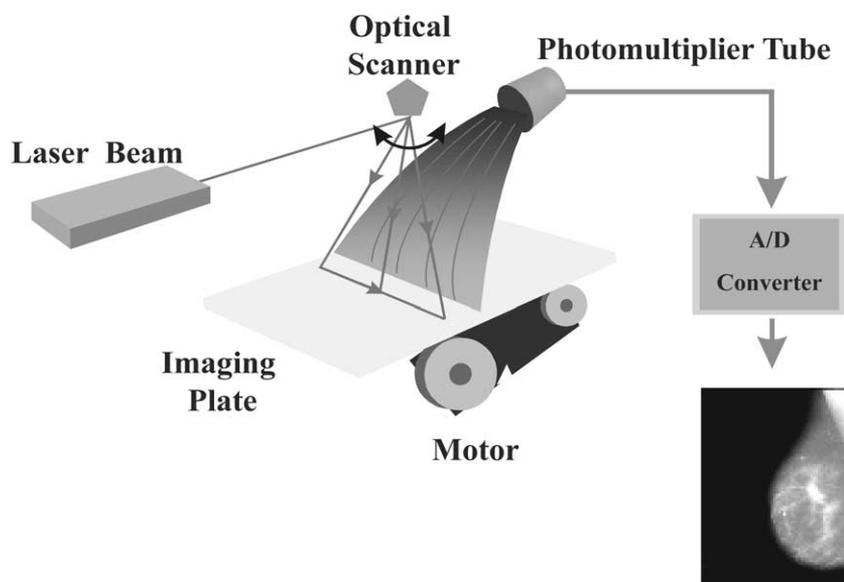
Fig 5. In CR, a laser scans the image plate from side-to-side, while a motor moves the plate under the laser. Light is emitted where x-rays stimulated the phosphor during the exposure. This process is called photostimulated luminescence. After readout, it is necessary to condition the plate before reuse (not shown). (Courtesy of Fuji Medical Systems, Stamford, CT.)
