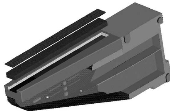
**Fig 7.** A computer representation of the scanning detector from the Fischer Senoscan digital mammography system. The detector consists of a phosphor screen (top), optical coupling element, and the optical sensor. The long narrow slot format allows the detector to be scanned across the breast quickly, thereby producing a high-quality image with a minimum of scatter. (Courtesy of Fischer Imaging, Denver, CO.)
