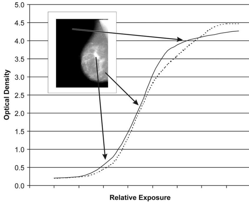
**Fig 1.** An example of the characteristic curves for 2 different modern, mammographic screen-film systems. For illustrative purposes, the different densities of a mammogram are mapped to regions of the Hurter and Driffield curve.
