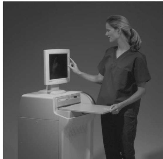
**Fig 4.** A picture of a compact, modern CR plate reader. (Courtesy of Fuji Medical Systems, Stamford, CT.)
