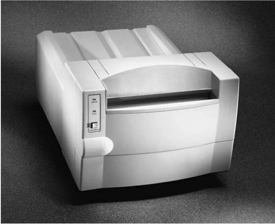
**Fig 3.** A picture of a laser film digitizer. A laser beam scans the film in 1 direction; the film is physically moved in the other direction. In this way, an image is constructed pixel by pixel. (Courtesy of Lumisys, Sunnyvale, CA.)
