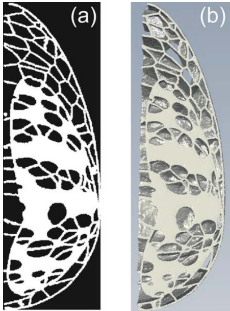
FIG. 3. (a) Tomographic slice of the voxel phantom composed of fibroglandular tissue, skin, and Cooper's ligament, corresponding to the slice of the voxel phantom shown in Fig. 1. (b) A 1 cm thick section of the voxel phantom ready for rapid prototyping.
